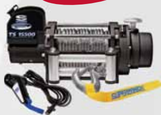
1515200 Tiger Shark 15500 Line Pull: 15,500lbs /12v Motor: Sealed 5.7 hp Wire rope: 29/64" x 94'
