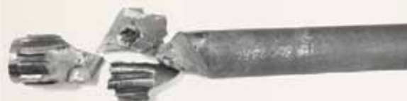
Land Rover OE Break Point 4800 Nm
