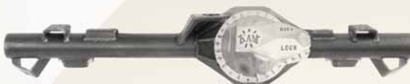
Rear axle tube with removable KAM Differential cover
