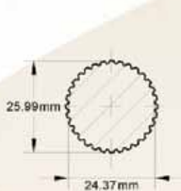
32 spline shaft cross section is 542mm sq.
