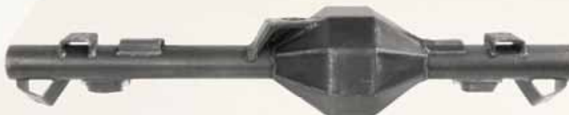
Rear axle tube with fully welded cover
